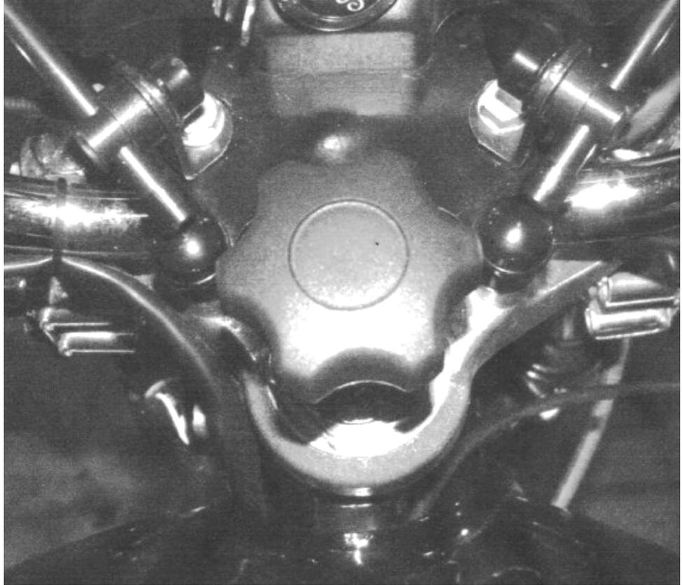
4. An M10 nutplate (see drawing) to be riveted or otherwise fixed to the underside of the lower plate of the existing steering damper assembly. (I had to make my own, as I couldn't find a commercially-available nutplate of this size. You might have more luck). To fix the nutplate, I used 5/32" x ¼" pop rivets. (left over from grafting a new pair of GRP front wings onto a Rover '90', back in the days when we did things like that!)
