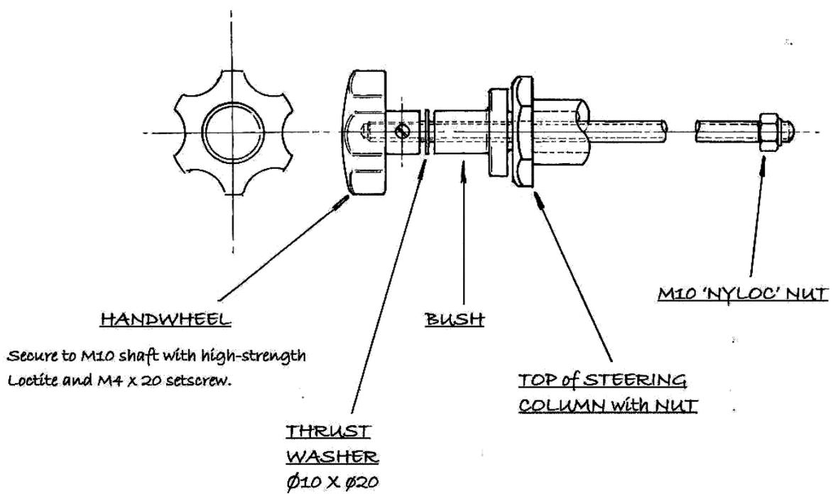
**ARRANGEMENT of STEERING DAMPER COMPONENTS**
